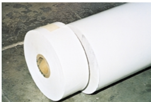
4. Narrow test rolls are sawn off the wide roll.
