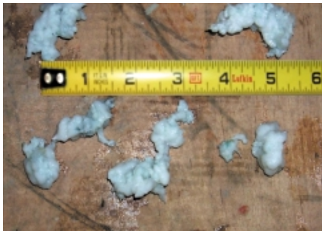
4. Example of "balled" PSA material
