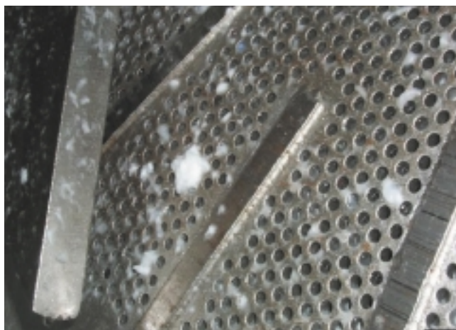
7. Detrasher interior: no PSA, no "balled" PSA evident
