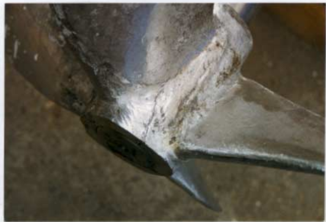
Figure 9. Cracks in 6-Mo side-entry agitator.
