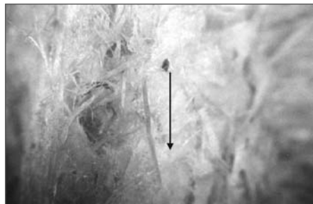
9. Inside view of the aggregate shown in Fig. 8. The fibers are aligned parallel to the breaker-bar (arrow) (4X).
