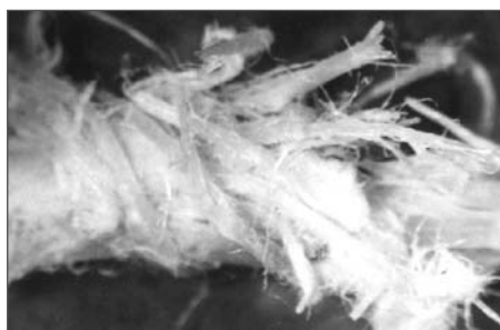
4. A rope-like strand of fiber bundles wrapped with defiberated elements collected from breaker-bar segment near refining zone (4X)
