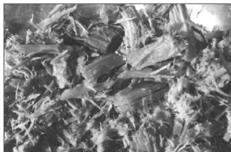
1. Chips from the feed-screw entering the refiner chamber. They are physically heterogeneous (0.4X)
