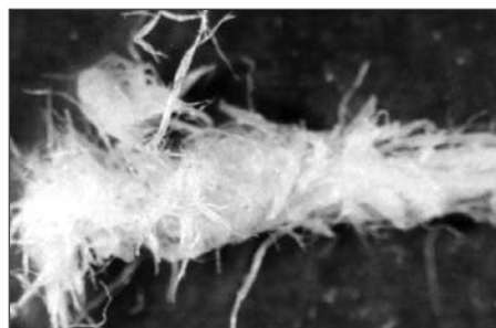
5. A strand-like aggregate consisting of fibers and fiber bundles wrapped with fiber elements collected from breaker-bar segment near refining zone (6X)
