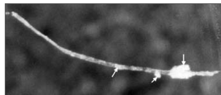
14. A single-fiber aggregate from the refiner discharge. The fiber is sporadically enwrapped with fines (arrows) (40X).
