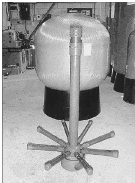
3. From the bottom of this feeder, water flows up through a bed of granular BrMEH. The water flow and temperature are controlled to dissolve biocide to the proper concentration.
