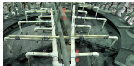
2. The gas sparged, cyclone-type (GSC) flotation cell was fitted with a bank of 14 nozzles for delivery of the surfactant spray onto the surface of the aerated pulp.
