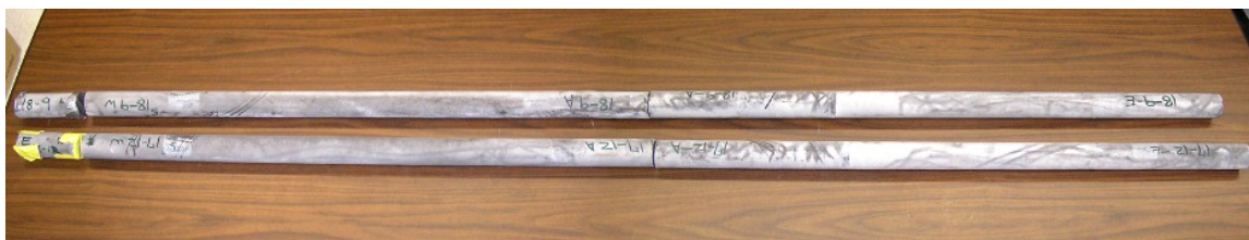
Figure 15. Heater tubes 17-12 and 18-9 that were taken from an area thought to be unaffected by overheating.
