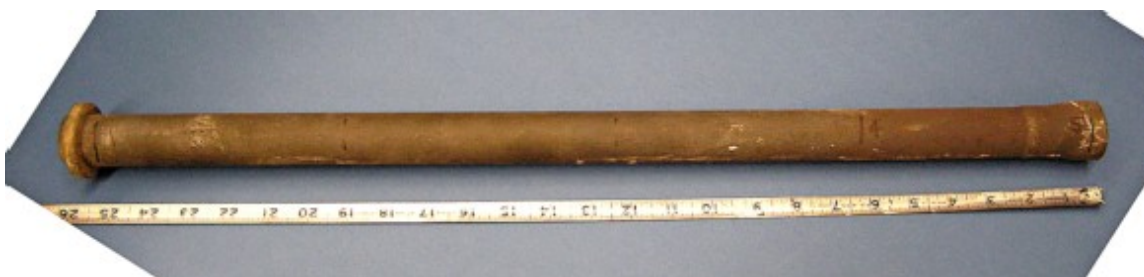
Figure 5. Shield tube from the mill in Trenton, Ontario, Canada. Note the flared exhaust end on the right and the collar on the left end that provides for mounting in the tube sheet.
