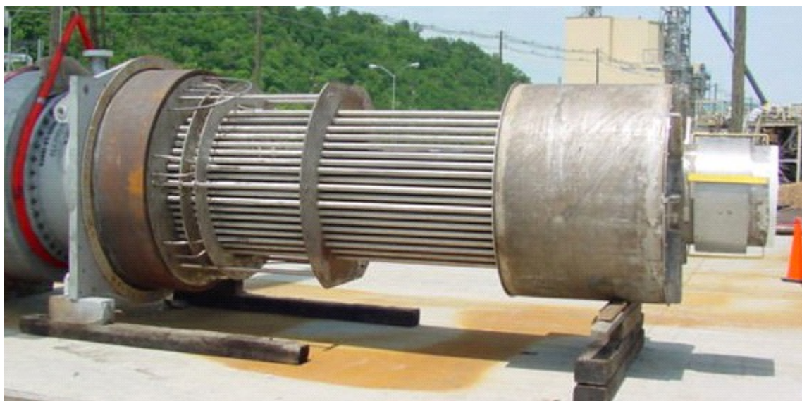
Figure 3. Pulse heater module showing the combustion chamber on the far left with the 253 heater tubes in the center and the exhaust plenum on the right.
