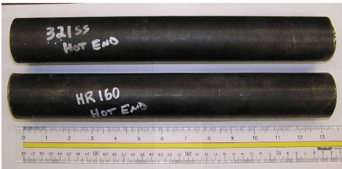
Figure 27. Photo of two sections of heater tube removed from the hotter end of the heater bundle.
