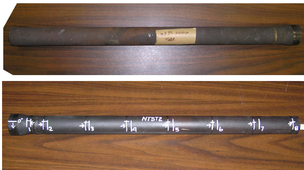
Figure 24. Photos of the as-received 330 stainless steel shield tube from the Trenton, Ontario, mill and the tube as marked for wall thickness measurements and preparation of metallographic samples.
