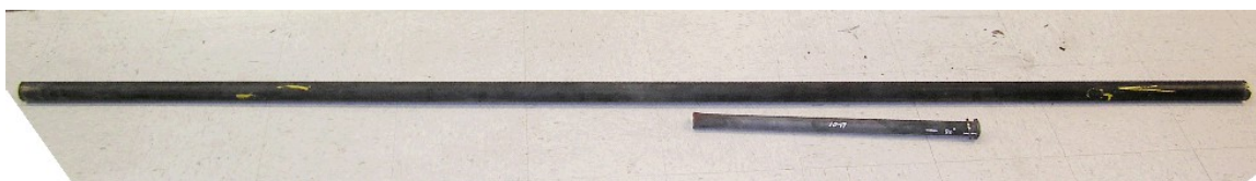
Figure 19. Pulse heater tube 10-17 with shield tube. The shield (shorter) tube is 66 cm (26 in.) long.
