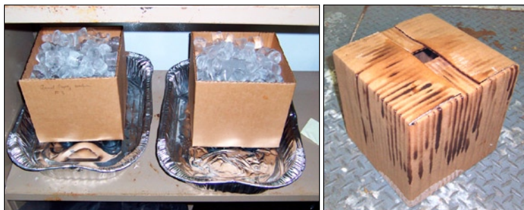
9. Photograph of the simulated end-use ice-pack test for waterproofing performance on the left, on the right, bottom of a box after 72 hours of ice-pack exposure showing wicking along the outside facings.
