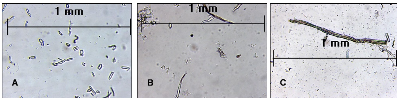
1. Optical micrographs of (A) primary fines from unrefined bleached hardwood kraft pulp, (B) secondary fines from refining of bleached hardwood kraft fibers, and (C) fibers obtained by repulping and fractionating unprinted xerographic copy paper.
