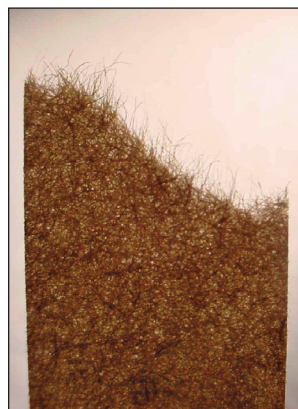
9. Tensile-test sample (grammage 60 g/m², width 15 mm) of the paper made from the fibrous fraction of the unbleached recycled kraft pulp. The rupture zone of the paper shows that many intact fibers were pulled out during the rupture.
