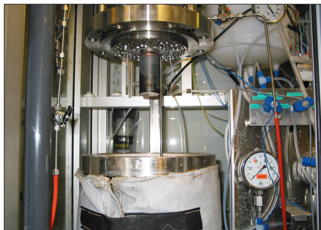
2. The autoclave, the lid of the autoclave, and the sensor fixed to the lid.
