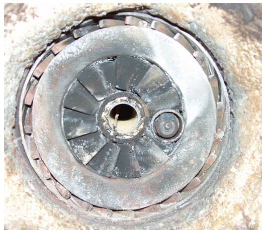
4. The figure at left shows the burner after test L2, where there was recirculation of lignin powder toward the hot burner surfaces. At right, some soot can be seen on the vanes of the secondary zone in test L3, but no clumps of char on either the primary or the secondary zone. The refractory lined cone is not shown in this figure.
