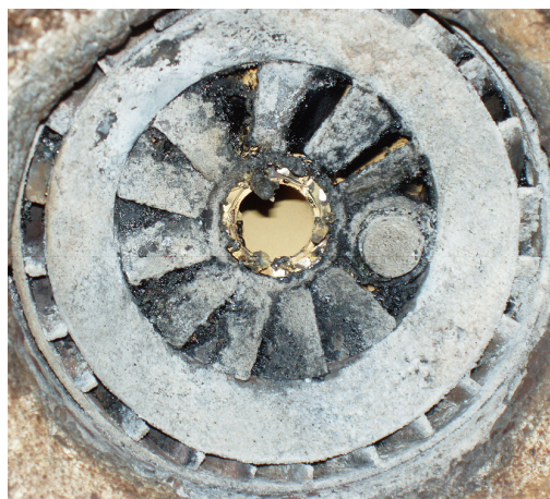
4. The figure at left shows the burner after test L2, where there was recirculation of lignin powder toward the hot burner surfaces. At right, some soot can be seen on the vanes of the secondary zone in test L3, but no clumps of char on either the primary or the secondary zone. The refractory lined cone is not shown in this figure.
