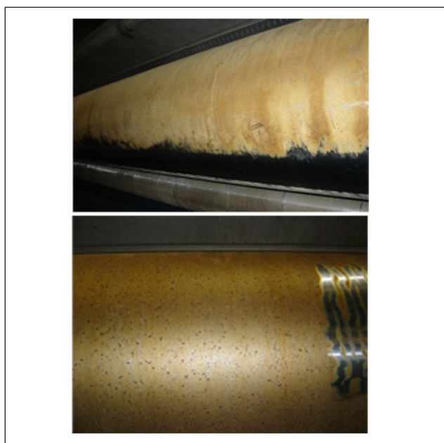
1. Pitch-related build-up on the guide roll of a supercalender.
