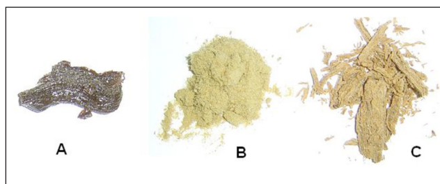
4. Appearances of build-up samples (A: control sample without pitch control strategy, B: with detackifier program, C: with the PAC program).
