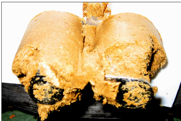
8. Homogeneous corn stover "paste" recovered after a TR test with CMC added.
