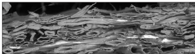
2. A scanning electron microscope (SEM) image of a CTMP lab sheet performed at Albany International.
