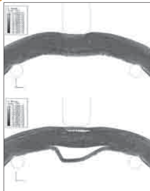
Delamination pattern after folding of a single ply sheet: a) the maximum ZD tensile strength is 275.6 kPa and maximum shear stress is 5512 kPa; b) the maximum ZD tensile strength is 689 kPa and maximum shear stress is 2756 kPa.
