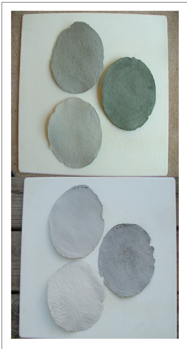
4. Counterclockwise, from top: pulped, floated, and reject pads of flexographic-printed (top photo) and inkjet-printed (bottom photo) newsprint.
