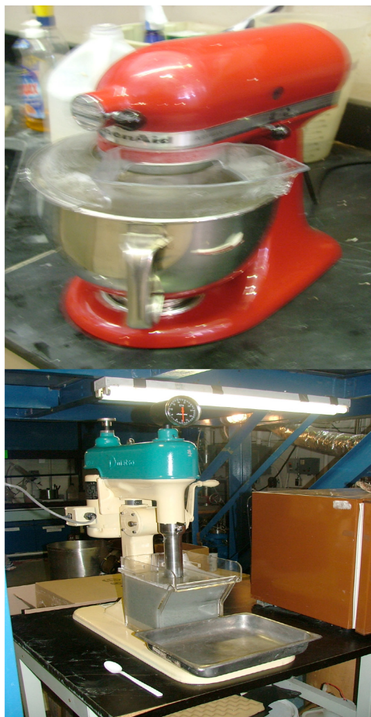
1. Mixer and Denver D12 laboratory flotation machine.
