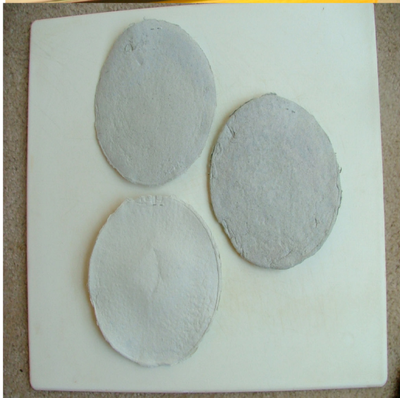
3. Counterclockwise, from top: pulped, floated, and reject pads of old newsprint (ONP).
