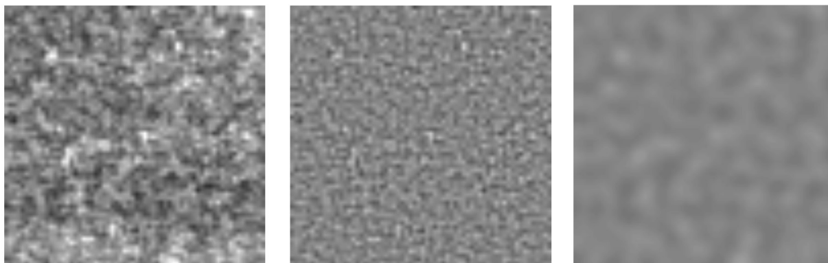
1. Original image (left) and two fast Fourier transform band passed filtered images of coating 1. The original image had a coefficient of variation size class 0-1 mm and had a coefficient of variation of 1.03% while the right image was in the size class 2-3 mm and had a coefficient of variation of 0.33%. In these images, the refractive index of pure black was 1.30 and of pure white was 1.43.
