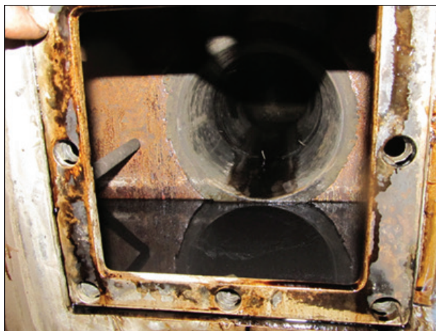
7. Upper MCC flow channel. (Nozzle height leaves 2.5 in. “heel” of liquor in the bottom).
