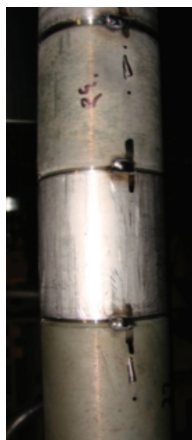
1. Schematic of the corrosion samples (left); photo of samples tack welded with thermocouples protruding from the surface of the samples (center); and photo of samples welded together and with shim stock welded in place to hold thermocouples on the surface of the samples (right).
