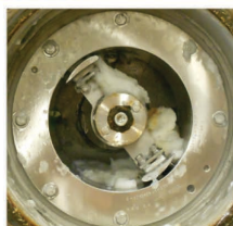
Front view of the screen cylinder and the EP foil rotor
