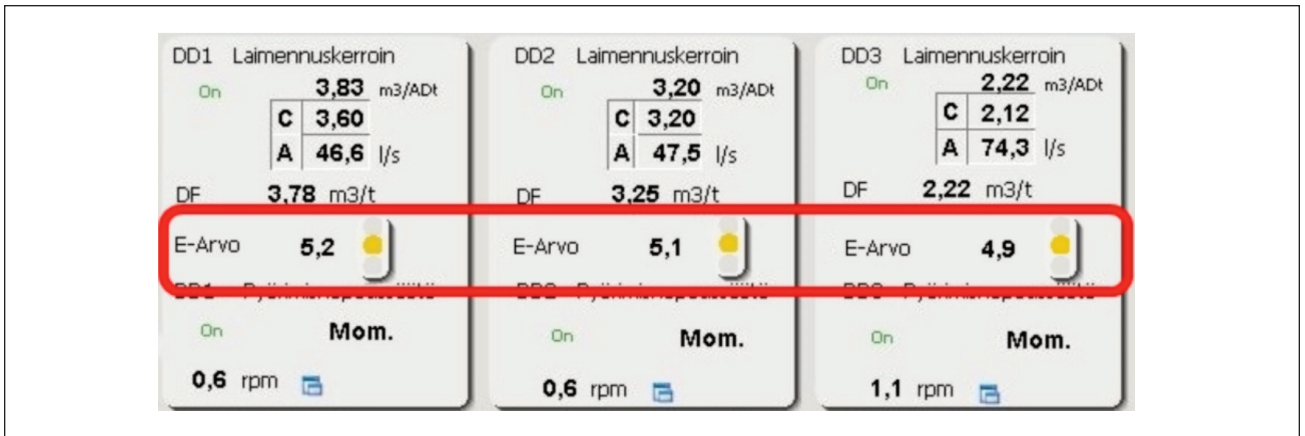
12. E-value and efficiency traffic lights on the operation monitor of the upper level control.
