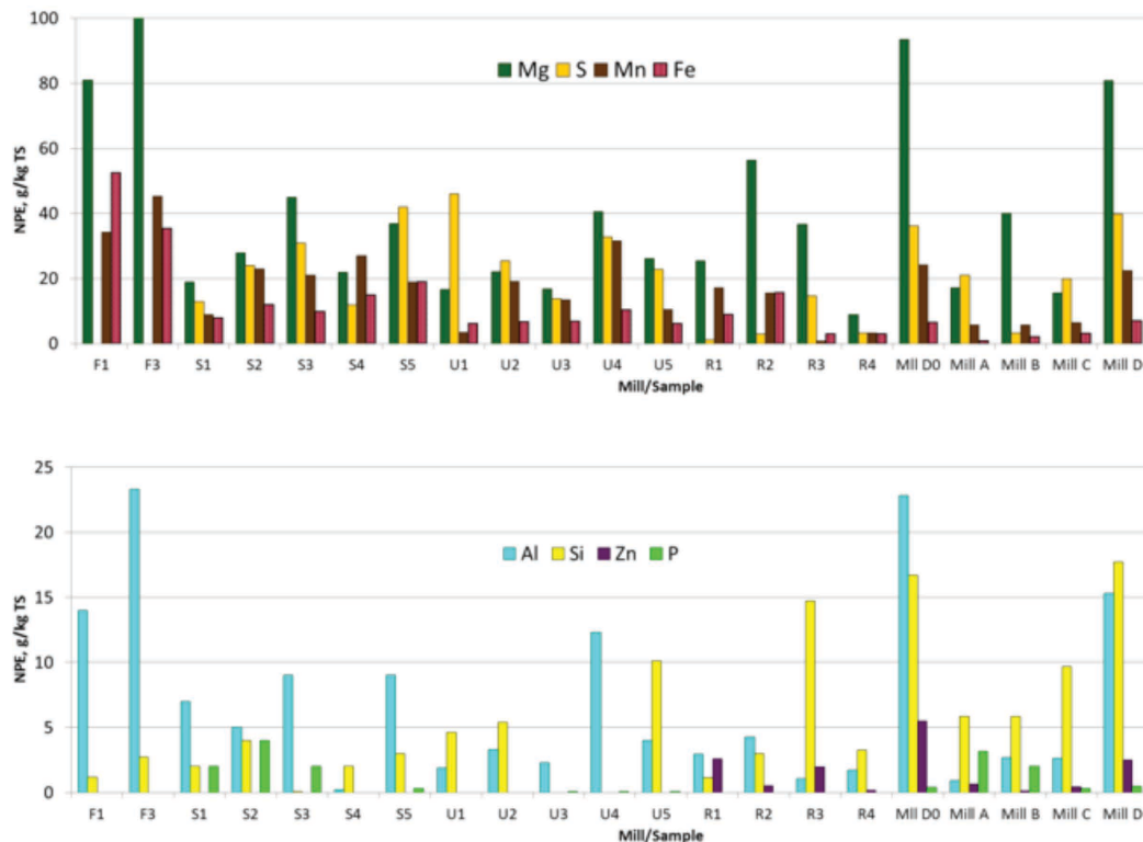
4. NPE levels in green liquor sludge (F1-F3, S not analyzed; S1-S5 and U1-U5 [11]; R1-R4 [7]; Mill D0, previous work; Mill A-Mill D, this work).
