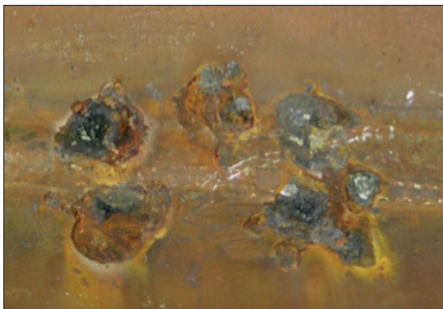
8. Heat exchanger 1: Pits under deposit mounds on the water-side of the cooling water discharge nozzle.
