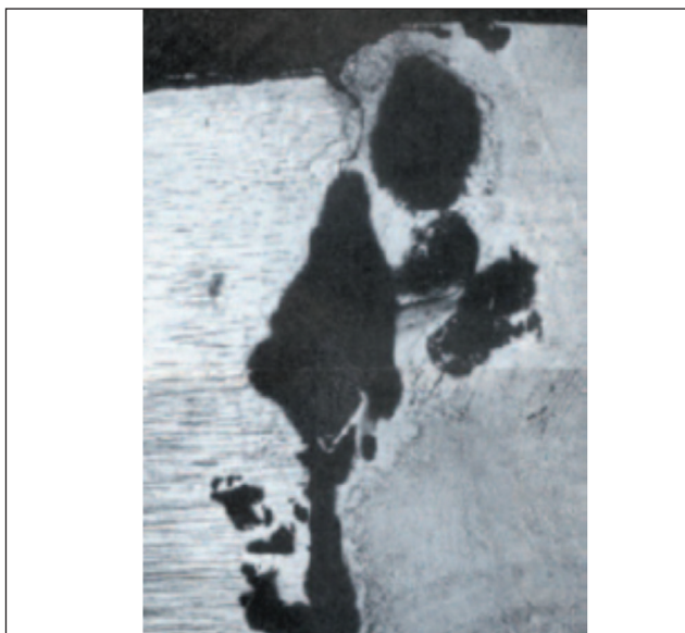
16. Rounded subsurface pits along a weld joining two adjacent lining sheets.
