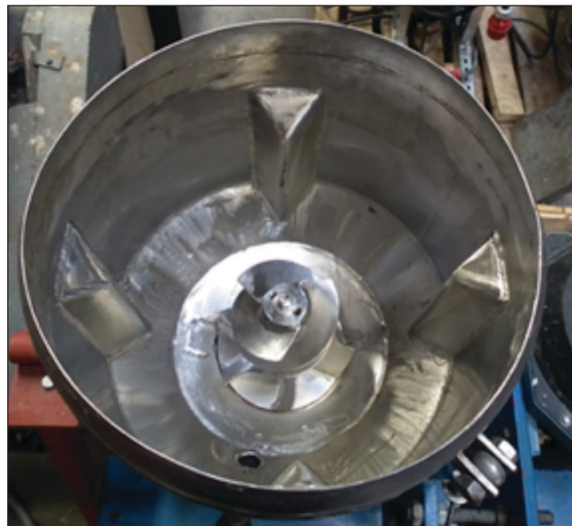
2. Low consistency pulping system ( h = 280 mm and Ø = 400) mm with helical rotor (rotor h = 170 mm); rotor speed = 1450 rpm.
