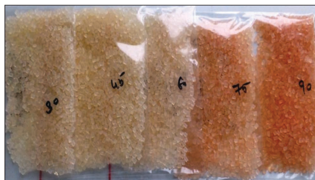
20. Polyamide granules after granule-assisted dispersion at 20% consistency with temperature from 30°– 90°C.
