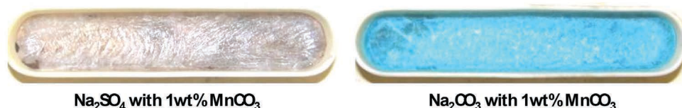
13. Appearance of pure \text{Na}_2\text{CO}_3 or \text{Na}_2\text{SO}_4 mixed with 1 wt% \text{MnCO}_3 after being heated at 920^\circ\text{C} for 30 min in air.
