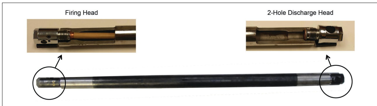
8. Photograph of 50 mm outer diameter (O.D.) x 1.25 m long \text{CO}_2 gas cartridge showing the firing and discharge heads. A 2-hole discharge head is shown here. A four-hole discharge is also available. Both the two- and four-hole designs work well to dislodge kiln rings.
