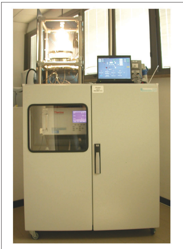
4. The photodegradation kinetics of nitrogen oxides (NO x ) in gaseous phase by foam-coated papers were tested using a photoreactor equipped with chemiluminescence and gas chromatography-mass spectrometry.
