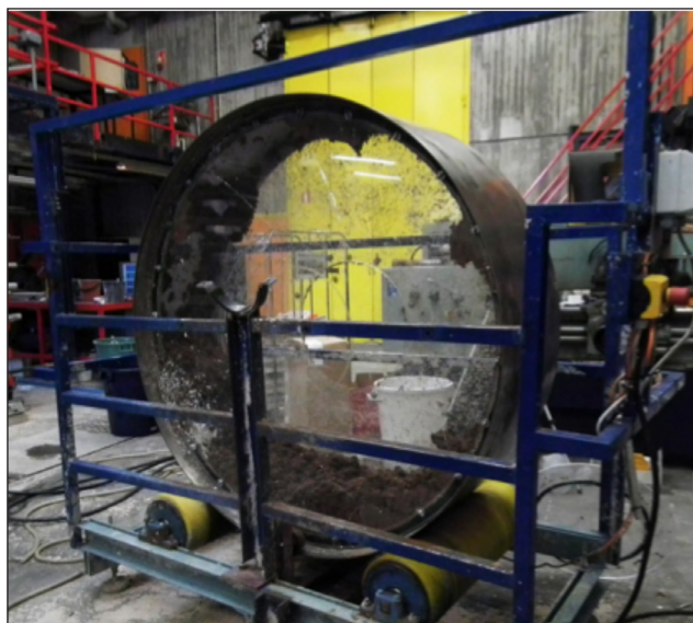
1. Drum pulper with 1.5 diameter, 8 lifters, and 10 cm lifter size.
