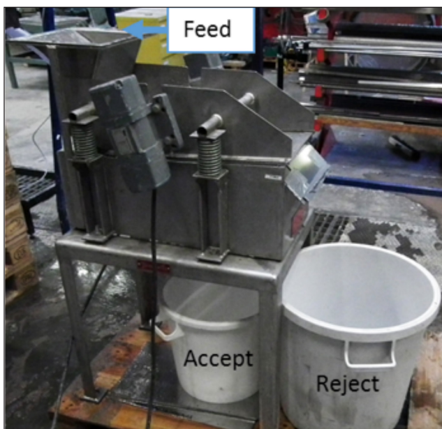
3. Tampella oscillating screen (Ø 4 mm). The feed sample was divided into reject (flakes) and accept (disintegrated pulp) samples. For all fractionations, feed consistency was adjusted to 0.5%.
