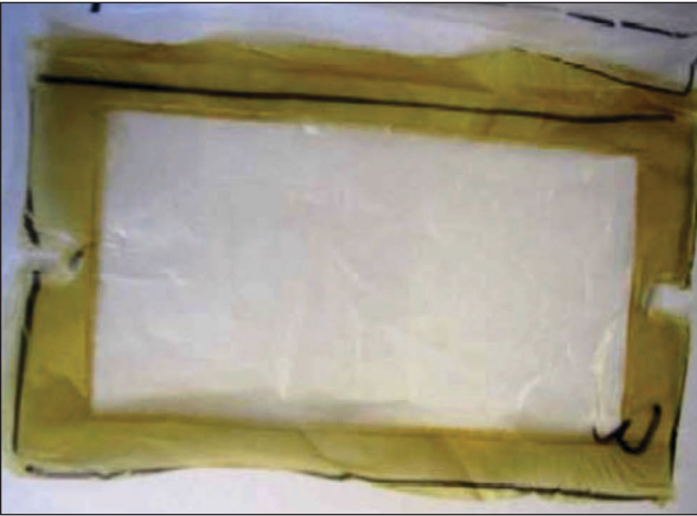
9. Hydroxypropyl lignin-containing polyester film (12–14 μm) following photo-irradiation in test chamber illustrating the photo-bleaching effect in the exposed film area. The fringe area remained shaded by clamping.
