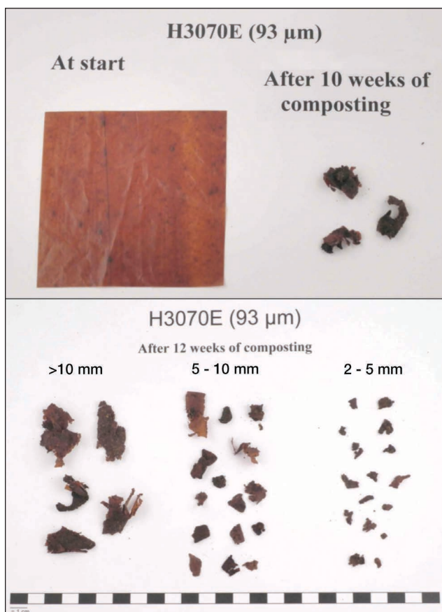
7. Illustration of the results of simulated composting tests with 93 µm-thick films. H3070E refers to sample designation by the contractor (Organic Waste Systems).
