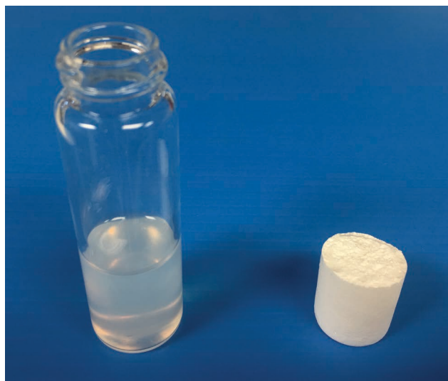
Current studies by L. Liang and A.J. Ragauskas are directed at designing lightweight nanocellulosic foams.
