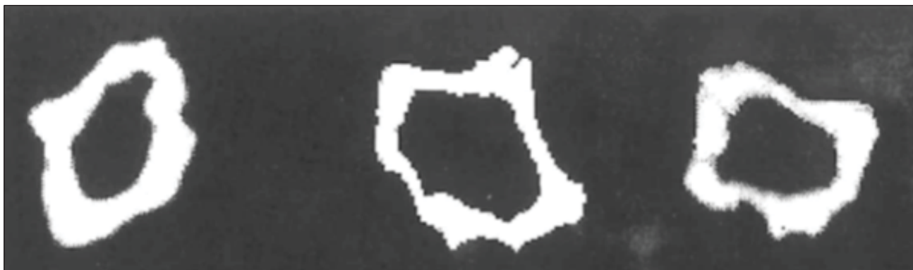
2. Confocal images of one typical fiber's cross section, determined by the method of Xu et al. [29]. From three measurements, the average wall thickness was determined to be 3.1 \mu\text{m} \pm 10\% , an equivalent diameter of 25 \mu\text{m} , and a cross-sectional area of 190 \mu\text{m}^2 .
