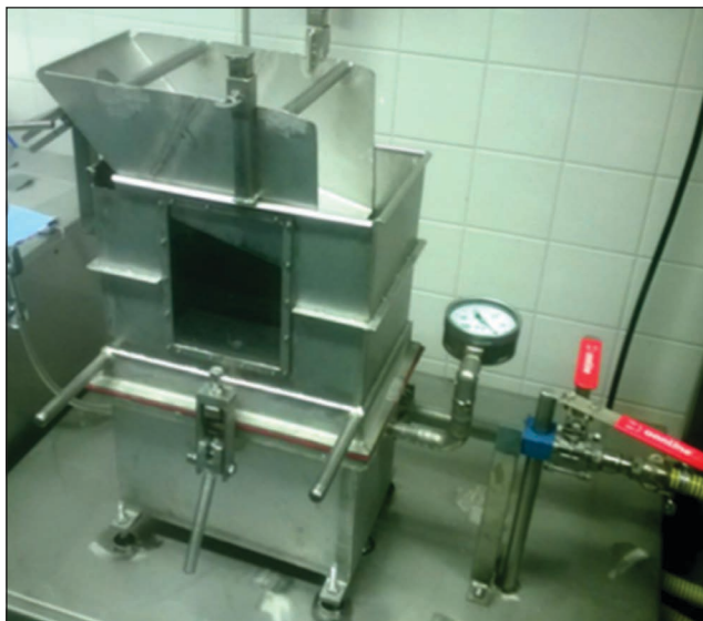
3. The foam forming handsheet mold with one-sided dewatering.
