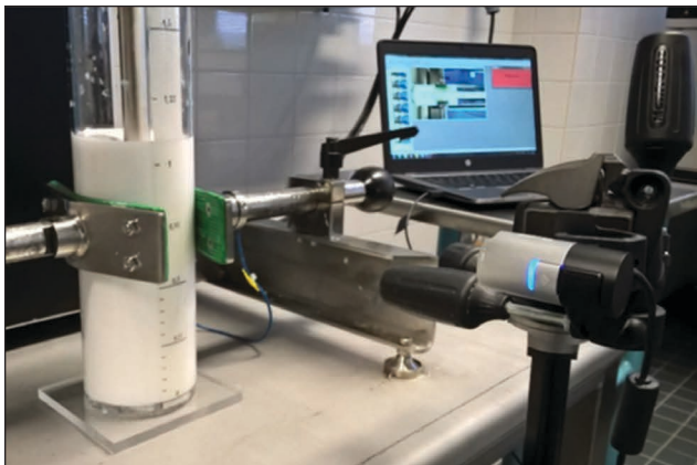
2. (a) The foam was produced in a mixer, and foaming dynamics were recorded with a charge-coupled device (CCD) camera. (b) Determination of bubble size distribution of the fiber-foam mixture.
