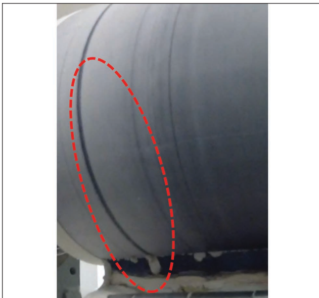
5. Wet bleeding with possible slip plane failure at the roll surface with K90 at a solids concentration of 59.43% and a roll speed of 360 m/min.
