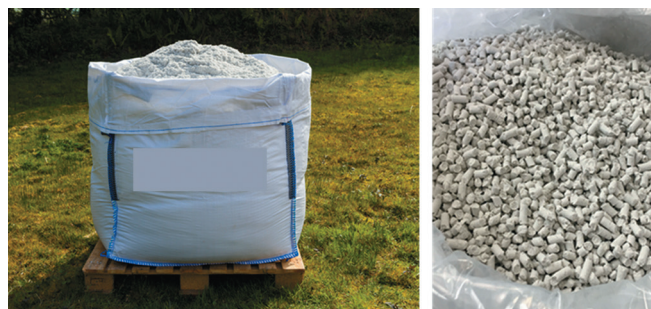
High solids mineral/MFC composite products prepared at full production scale.
