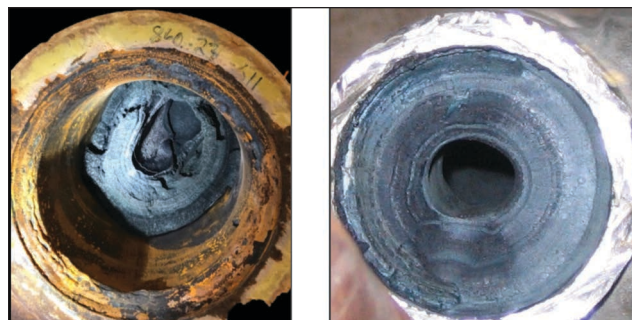
1. Calcite ( \text{CaCO}_3 ) scale formation in green liquor pipelines at two kraft mills. Pipe inner diameter = 8 in. (20.3 cm) in both cases.
