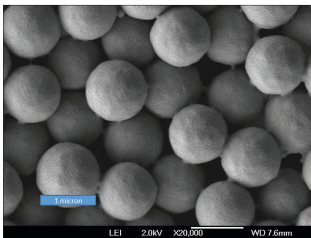
1. Surface scanning electron microscope (SEM) image of the HSP4 hollow sphere pigment (HSP).
