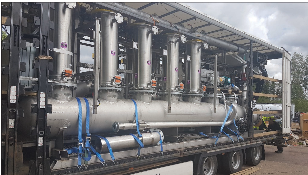
11. Skid for the Ence Pontevedra mill's patented CleanFlow system.
