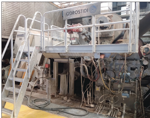
1. Rod sizer-spooner section of a papermaking machine.
