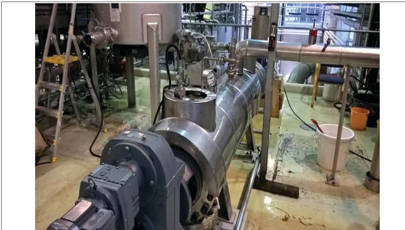
2. Pilot-size continuous screw reactor. Length of the reactor vessel is approximately 2.2 m, and the inner diameter is 0.34 m.
