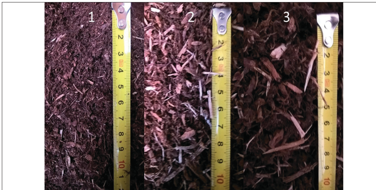
4. Three fractions obtained by use of the vibrating slope screen.
