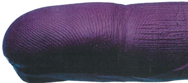
Artificial finger to evaluate the touch of fabrics resulted from a multidisciplinary approach. (Source: S.S. Ramkumar, Ph.D. studies, 1998, University of Leeds, UK.)
