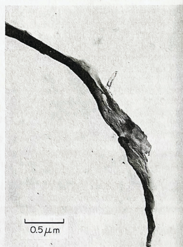
Fig. 5. Cell wall fragment of sprucewood meal after delignification. Platinum-shadowed.
