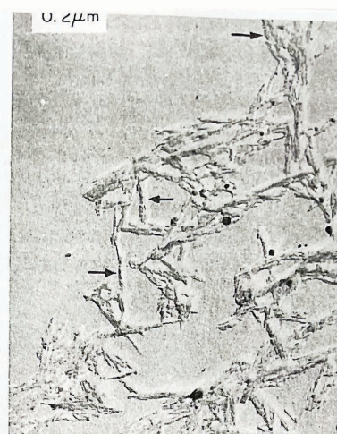
Fig. 8. Partially hydrolyzed cellulose (20% \text{H}_2\text{SO}_4 , 5 hr, 100^\circ\text{C} ) from sprucewood. The fibrillar fragments are subdivided in longitudinal direction (arrows). Platinum-shadowed.
