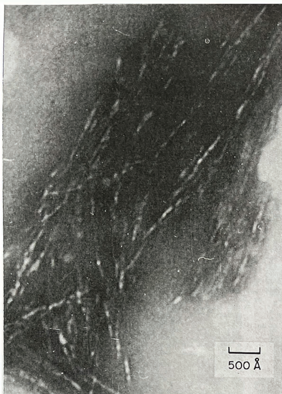
Fig. 9. Partially hydrolyzed cellulose (20% \text{H}_2\text{SO}_4 , 5 hr, 100^\circ\text{C} ) from sprucewood. The fibrillar elements have a beaded appearance. Negative stained with phosphotungstic acid (PTA).
