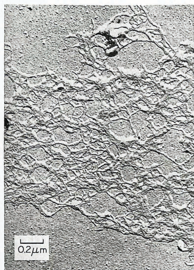
Fig. 1. Polyose Fraction A2 from beechwood containing fibrillar xylan. Platinum-shadowed.
