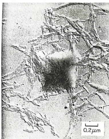
Fig. 6. Partially hydrolyzed cellulose (20% \text{H}_2\text{SO}_4 , 5 hr, 100^\circ\text{C} ) from sprucewood. The fibrillar fragments are arranged in various lateral aggregates. Platinum-shadowed.
