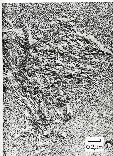
Fig. 14. Partially hydrolyzed cellulose (20% H_2SO_4 , 1 hr, 100°C) from sprucewood. Newly formed fibrillar systems. Platinum-shadowed.
