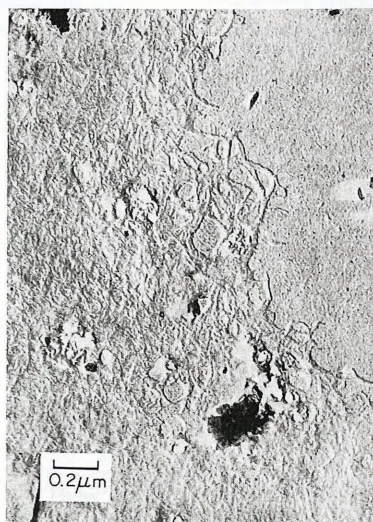
Fig. 2. Polyose Fraction A2 from sprucewood containing fibrillar arabinoxylan and amorphous-looking glucomannan. In several places, the smooth areas are resolved into fine fibrillar structures. Platinum-shadowed.
