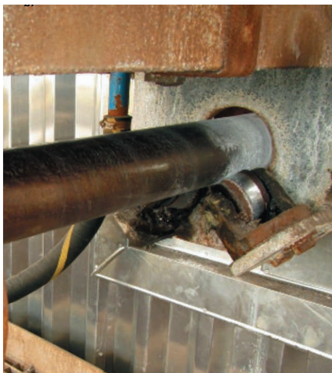
Lance support rollers should freely turn to avoid external mechanical damage.
