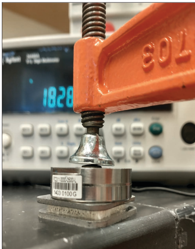
1. Screw press used for dewatering trials. Shown from bottom to top: the bottom platen, paper, press felt, top platen, force sensor, and screw press.
