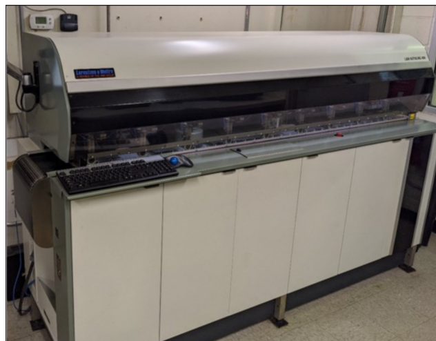
1. ABB L&W Autoline automated paper and board testing system used by the Alsip MiniMill.
