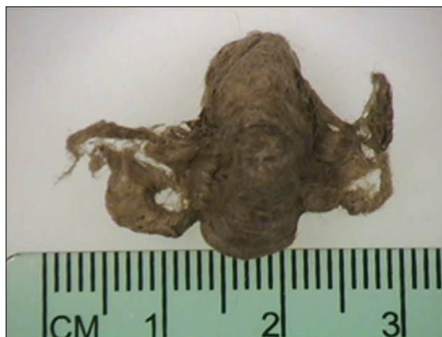
6. Strings removed from the base headbox.
