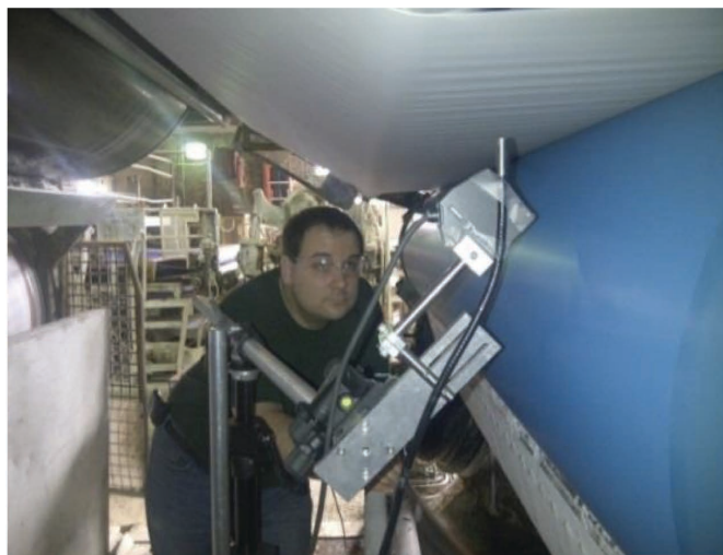
3. Portable infrared moisture sensor positioned in the open draw of a commercial fine paper machine. Shown also is the effect of distance between the sensor and paper surface on moisture measurement.
