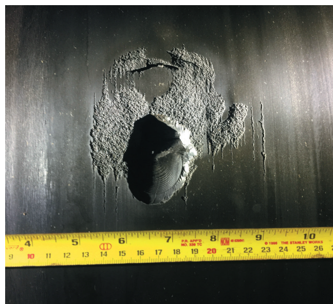
Damage to roll cover from vibration when nip load went roughly double the design nip load, result in removal of rubber from the cover.
