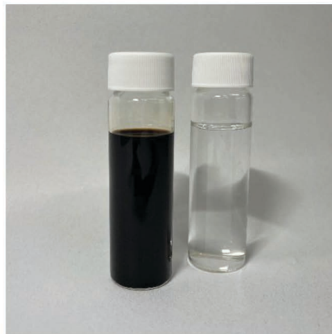
8. (a) Chemical characterization of the membrane permeate and a combined condensate sample from the same mill, and (b) a picture of the feed black liquor (left) and the output permeate (right). The permeate is visibly clear and of comparable composition to the combined condensate.
